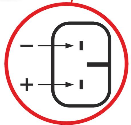
DURING THE TEST OPERATIONS OF THE SCROLL TYPE A/C COMPRESSOR WITH EXTERNAL ELECTRICAL POWER SUPPLY IT IS **NECESSARY CHECK CAREFULLY THE CORRECT POSITION OF THE CONNECTOR (SEE PICTURE ABOVE)**. THE COMPRESSOR MUST BE POSITIONED WITH HOSE MANYFOLD TOWARD UP, IF THIS CHECK IS NOT RESPECTED YOU CAN CREATE AN ELECTRICAL SHORT-CIRCUIT AND ITS DAMAGING.
